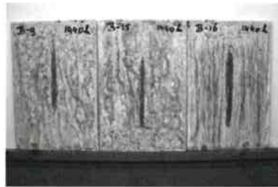
ZINGA 2 x 90 µm DFT after 1440 h salt spray.
