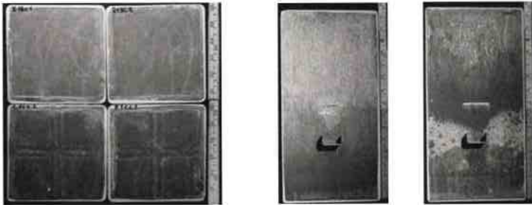
ZINGA 2 x 60 µm DFT after 180 days in a condensation chamber (left) or a wave tank (right)
